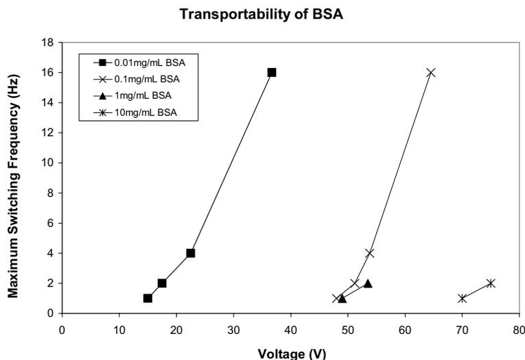
**Figure 3 – Maximum switching frequency of BSA droplets as a function of voltage for various concentrations.**
